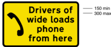
7293 Instructions to drivers of wide loads on location from which they should telephone for assistance
