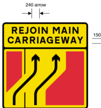
7231 Return of traffic from hard shoulder and left lane of carriageway to left and centre lanes
