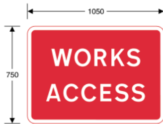
7301 Temporary access to a construction or road works site
