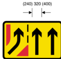
7254 Additional traffic lane joining from the left at a junction as part of temporary traffic management scheme
