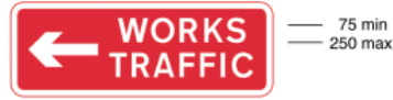
7304 Direction to be taken by road works or construction traffic at a junction or works entrance ahead
