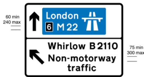
2124.1 Junction ahead of a non-primary route which leads directly onto a motorway, with another non-primary route which should be followed by traffic not wishing or permitted to use the motorway
