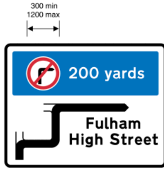
2123 Distance to a prohibited movement and direction to the destination shown avoiding that prohibition
