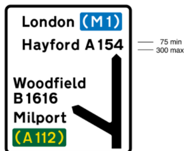
2101.2 Grade separated junction of a non-primary route leading to a motorway with another non-primary route leading to a primary route
