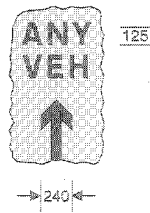
7281 Symbol that may be incorporated into a road works sign to indicate a lane open to any vehicle
