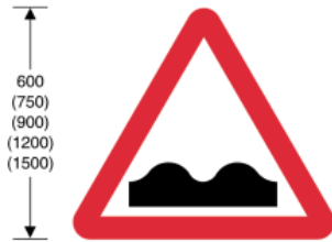
556 Uneven road ahead
