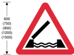
529 Opening or swing bridge ahead
