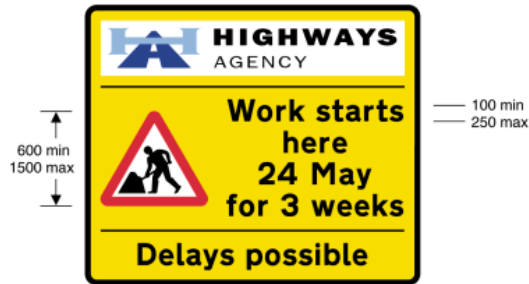
7003.1 Starting date and duration of road works
