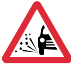
7009 Loose chippings on road ahead
