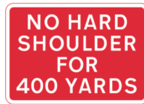
7015 Temporary absence of hard shoulder for distance specified
