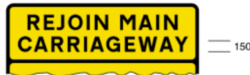
7261 Panel to appear at top of road works sign instructing traffic using hard shoulder to rejoin main carriageway
