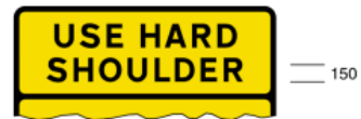
7260 Panel to appear at top of road works sign allowing traffic to use hard shoulder as indicated on main part of sign
