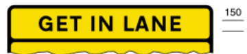
7262 Panel to appear at top of road works sign instructing traffic to get into the appropriate lane as indicated on main part of sign
