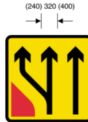
7255 Additional traffic lane available ahead as part of temporary traffic management scheme
