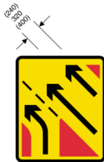
7251 Additional traffic lanes joining from the right at a junction as part of temporary traffic management scheme
