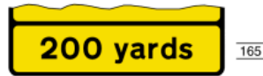
7271 Panel to appear at bottom of road works sign indicating distance in yards to point at which condition indicated by signs shown in diagrams in item 3 of the table start to apply
