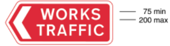
7305 Direction to be taken by road works or construction traffic at a junction or works entrance
