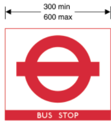
973.2 Stopping place for buses operated by or on behalf of or under agreement with Transport for London
