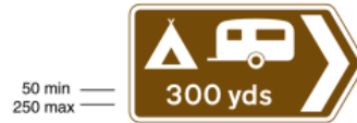
2302 Direction and distance to a camping and caravan site as defined in the caption under diagram 2301
