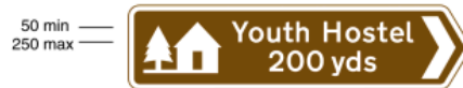
2304 Direction and distance to a hostel as defined in the caption under diagram 2303
