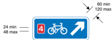
2601.1 Direction of a numbered route for pedal cycles forming part of a national cycle route network at a junction ahead
