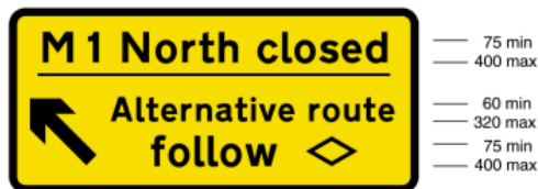
2716 Junction ahead leading to a temporary diversion route, the direction along which is indicated by a symbol shown in Part VII of Schedule 13
