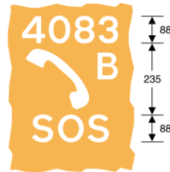
2715 Back of emergency telephone box
