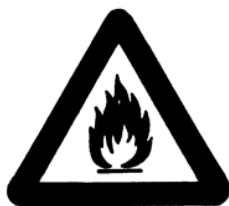
Flammable material or high temperature (1)
