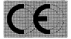
If the CE marking is reduced or enlarged the proportions shown in the above drawing must be respected.
