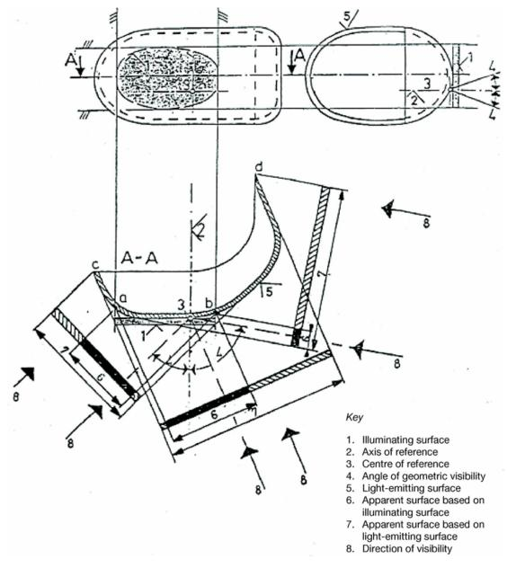
NB: Notwithstanding the drawing the apparent surface is to be considered as tangent to the light-emitting surface.
