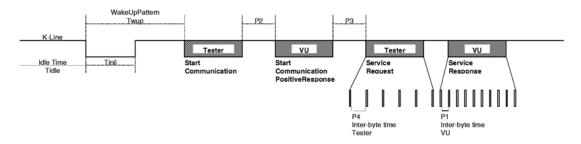
The timing values for the fast initialisation and communications in general are detailed in the tables below. There are different possibilities for the idle time:
