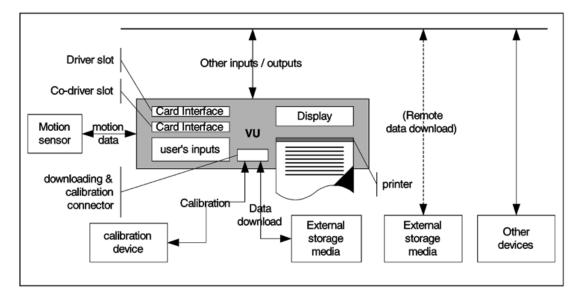
The VU general characteristics, functions and mode of operations are described in Chapter II of Annex I B.
