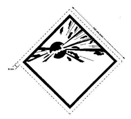
(b) comply with the measurements in the diagram, except that larger measurements may be used in which case the measurements shall be increased proportionally.
