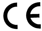
The different elements of the EC mark should have materially the same vertical dimensions, which should not be less than 5mm.
