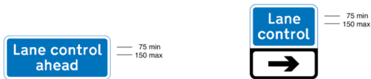
5012 System of lane control light signals ahead
