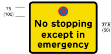
642.3 No stopping in lay-by except in emergency
