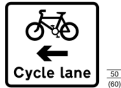
962.1 Cycle lane on road at junction ahead or cycle track crossing road
