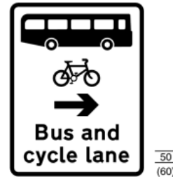
962.2 Contra-flow bus lane which pedal cycles may also use on road at junction ahead
