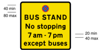
975 Place where buses may stand and the stopping of other vehicles is prohibited during the period indicated
