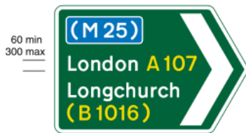
2026 Direction to a primary route which leads to a motorway and a non-primary route
