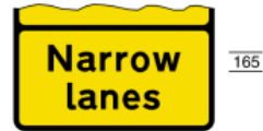
7274 Panel to appear at bottom of road works sign indicating that traffic lanes are narrower than normal
