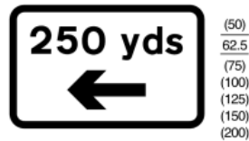
573 Distance and direction to hazard
