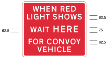
7027 Same as diagram 7011 where vehicles are to be escorted in convoys through road works
