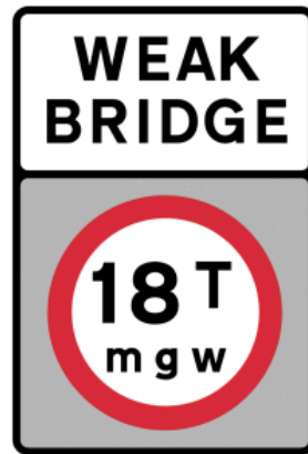
626.2A Vehicles exceeding the maximum gross weight indicated prohibited from crossing the bridge or other structure
