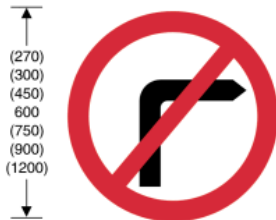
612 No right turn for vehicular traffic
