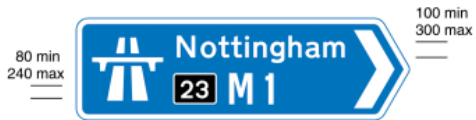
2902 Direction to a motorway at the junction shown, indicating route number and destination reached along the motorway
