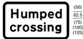
547.8 Zebra crossing or signal-controlled crossing on road hump ahead
