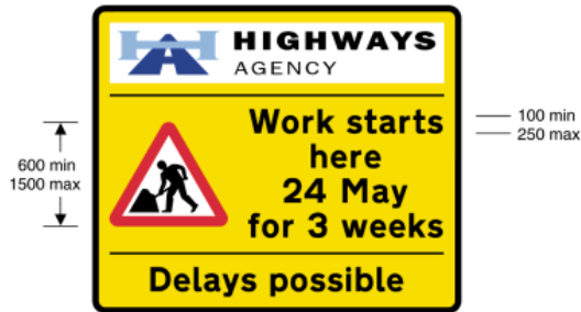
7003.1 Starting date and duration of road works
