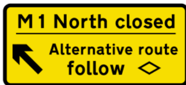
2716 Junction ahead leading to a temporary diversion route, the direction along which is indicated by a symbol shown in Part VII of Schedule 13
