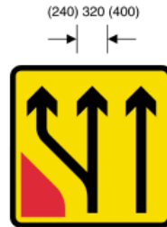
7255 Additional traffic lane available ahead as part of temporary traffic management scheme
