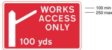
7306 Direction to be taken by road works or construction traffic to an access to a works site ahead
