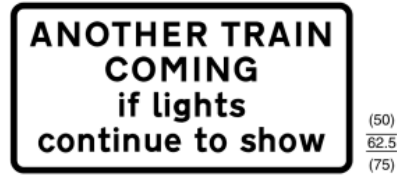
777 Level crossing ahead is crossed by more than one railway or tramway track, and more than one train or tramcar may pass over it in quick succession
