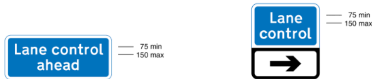
5012 System of lane control light signals ahead
