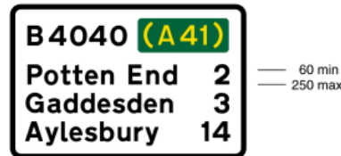
2128 The number of a non-primary route leading to a primary route with destinations and distances
