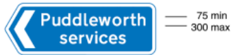
2311.1 Entrance or direction to a named motorway service area located on a road that is not a motorway (Sign on a primary or non-primary route)
