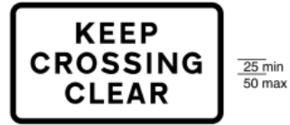
775 Vehicular traffic must not stop within the area of a railway or tramway level crossing
