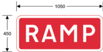
7013 Temporary sudden change in level of carriageway surface
