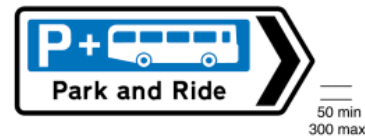
2504 Direction to a parking place from which a 'Park and Ride' scheme operates
