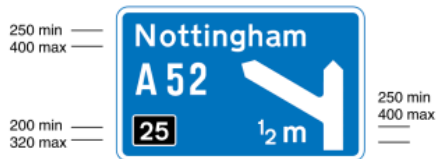
2903 Motorway junction ahead, identified by the number shown on a black background, leading to the destination and route shown. The number of lanes on the motorway remains the same through the junction
