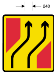
7237 Diversion of traffic from left and centre lanes to centre and right hand lanes
