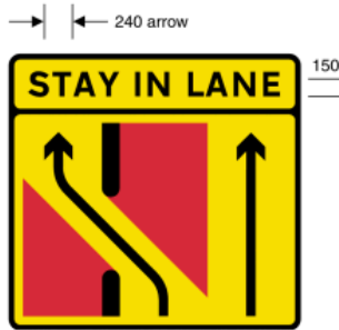
7218 Left hand lane returns from other carriageway to original carriageway ahead; right hand lane continues on other carriageway
