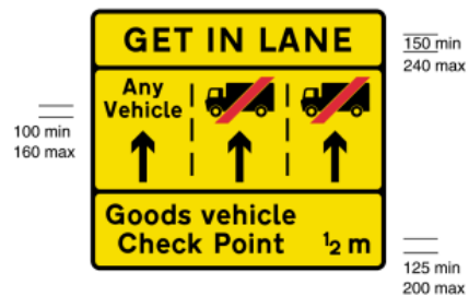
832.7 Goods vehicles should get into the left hand lane of a three lane carriageway on the approach to a goods vehicle check point ahead
