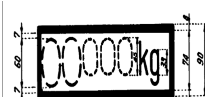
Fig. B2 Marking for the tare weight and braked weight of wagons fitted with handbrakes. U.K.
