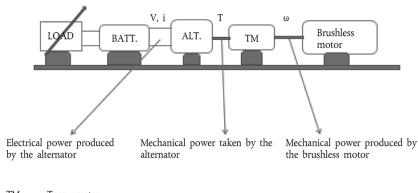
$\begin{array}{lll} TM &=& Torquemeter \\ ALT. &=& Alternator \\ BATT. &=& Battery \\ V,I &=& Volt, \ current \\ T &=& Torque \\ \omega &=& Rotational \ speed \end{array}$
