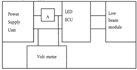
In total ten measurements is to be done with the following voltages: 9,0 V; 10,0 V; 11,0 V; 12,0 V; 13,0 V; 13,2 V; 13,4 V; 14,0 V; 15,0 V; 16,0 V (where values of 13,2 V and 13,4 V are typical values for the voltages in passenger's vehicles).
