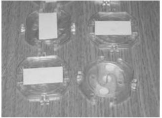
This case deals with socket protectors. These are devices that users (parents) put into the electrical socket outlets to stop small children from accessing live parts by putting a long metal object into one of the holes in the outlet and getting a (fatal) electric shock.
