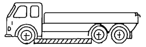
4.5.2. 'Ground clearance beneath one axle' means the distance beneath the highest point of the arc of a circle passing through the centre of the tyre footprint of the wheels on one axle (the inner wheels in the case of twin tyres) and touching the lowest fixed point of the vehicle between the wheels.
