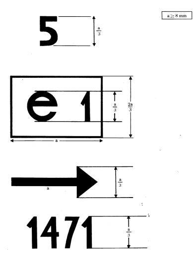
The device bearing the EEC component type-approval mark shown above is a direction indicator lamp in category 5 EEC type-approved in Germany (e 1) under the number 1471. The arrow shows in what position this device, which can be mounted only on one side of the vehicle, is to be mounted. The arrow points towards the front of the vehicle.
