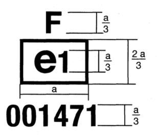
The device bearing the EC component type-approval mark shown above is a rear fog lamp, type approved in Germany (e1) pursuant to this Directive (00) under the base approval number 1471.
