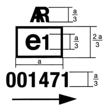
The device bearing the EC component type-approval mark shown above is a reversing lamp, type approved in Germany (e1) pursuant to this Directive (00) under the base approval number 1471. The arrow indicates the side on which the required photometric specifications are met up to an angle of 45° H.
