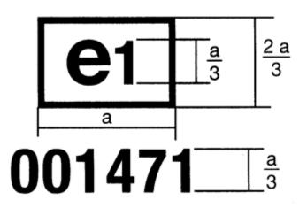
The device bearing the EC component type-approval mark shown above is a parking lamp, type approved in Germany (e1) pursuant to this Directive (00) under the base approval number 1471.]
