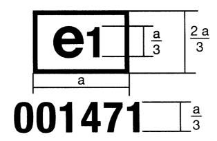
The device bearing the EC component type-approval mark shown above is a parking lamp, type approved in Germany (e1) pursuant to this Directive (00) under the base approval number 1471.
