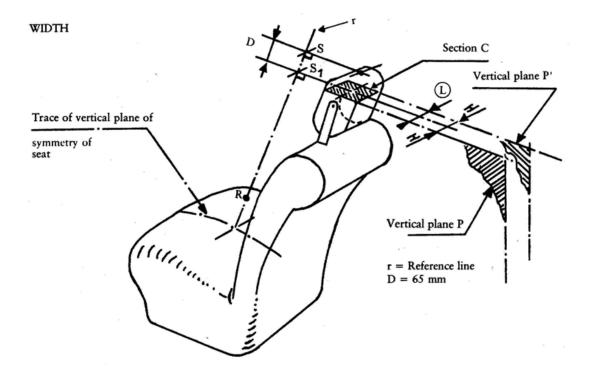
ANNEX IV DETAILS OF LINES DRAWN AND MEASUREMENTS TAKEN DURING TEST
