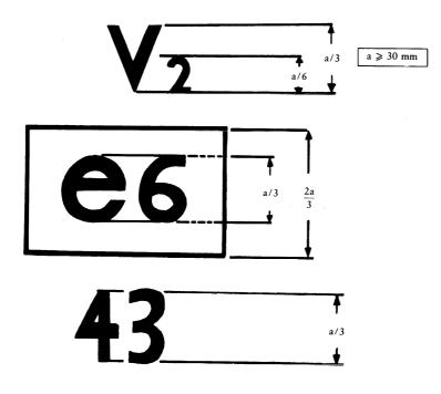
*Legend:* The protection structure bearing the EEC component type-approval mark shown above is a structure of the bar type subjected to a dynamic test with two front-mounted uprights intended for a narrow-track tractor (V2), for which EEC component type-approval was granted in Belgium (e6) under the number 43.
