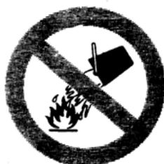
Do not extinguish with water
