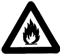
Flammable material or high temperature (1)
