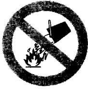
Do not extinguish with water
