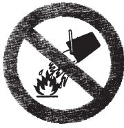
Do not extinguish with water
