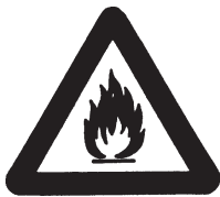
Flammable material or high temperature (1)
