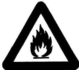
Flammable material or high temperature (1)
