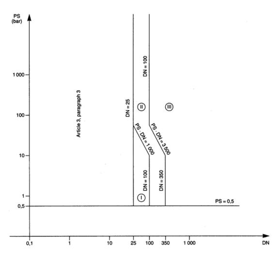
Exceptionally, assemblies intended for generating warm water as referred to in Article 3, Section 2.3, must be subject either to an EC design examination (Module B1) with respect to their conformity with the essential requirements referred to in Sections 2.10, 2.11, 3.4, 5 (a) and 5 (d) of Annex I, or to full quality assurance (Module H).
