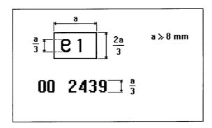
The above component type-approval mark shows that the combustion heater in question has been approved in Germany (e1) under approval number 2439. The first two digits (00) indicate that this component was approved according to this Directive.
