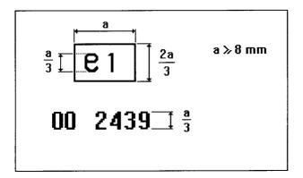
The above component type-approval mark shows that the combustion heater in question has been approved in Germany (e1) under approval number 2439. The first two digits (00) indicate that this component was approved according to this Directive.
