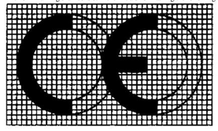
The 'CE' marking must have a height of at least 5 mm. If the 'CE' marking is reduced or enlarged the proportions given in the above graduated drawing must be respected.
