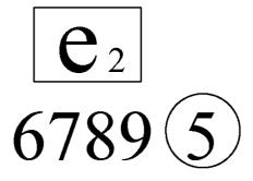
The above represented type-approval mark was issued by France [e<sub>2</sub>] under number 6789 for the replacement catalytic converter not integrated in the exhaust system (catalytic converter and silencer not integrated in a sole element) (see Chapter 5).
