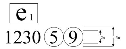
The above represented type-approval mark was issued by Germany  $[e_1]$  under number 1230 for a replacement catalytic converter consisting of a sole part integrating both the catalytic converter and the exhaust system (silencer).
