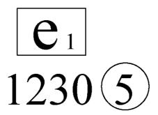
The above represented type-approval mark was issued by Germany [e<sub>1</sub>] under number 1230 for the replacement catalytic converter not integrated in the exhaust system (catalytic converter and silencer not integrated in a sole element).
