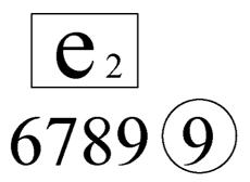
The above represented type-approval mark was issued by France  $[e_2]$  under number 6789 for a non-original silencer not integrating a catalytic converter (catalytic converter and silencer not integrated in a sole element or vehicle not equipped with a catalytic converter)
