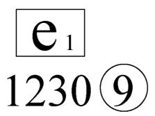
The above represented type-approval mark was issued by Germany [e<sub>1</sub>] under number 1230 for the non-original silencer not integrating a catalytic converter (catalytic converter and silencer not integrated in a sole element or vehicle not equipped with a catalytic converter) (see Chapter 9).'
