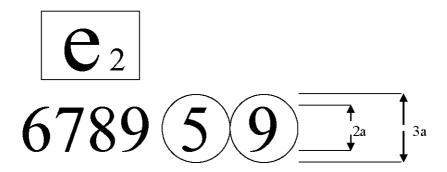
The above represented type-approval mark was issued by France  $[e_2]$  under number 6789 for a non-original exhaust system consisting of a sole part integrating both the silencer and the catalytic converter.
