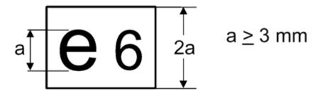
Legend: the above component type-approval was issued by Belgium under number 0004. 01 is a sequential number denoting the level of technical requirements to which this component fulfils. The sequential number is attributed in accordance with the relevant separate directive or regulation.
