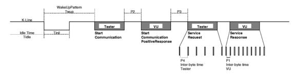
The timing values for the fast initialisation and communications in general are detailed in the tables below. There are different possibilities for the idle time:
