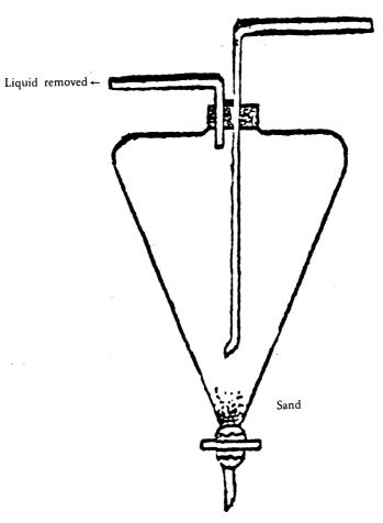
Diagram of apparatus used for continuous separation of water-insoluble mineral impurities
