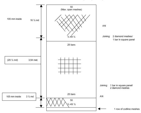
The construction of upper panel, size and position of the window panel in case when the escape panel runs from selvedge to selvedge
