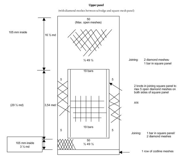
The construction of upper panel in case 20 % of diamond meshes in the upper panel are maintained and equally divided on both sides of the window.
