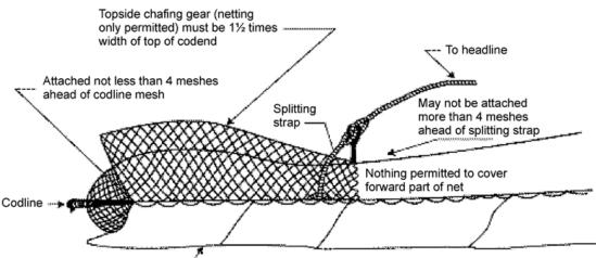
Chafing gear: Any material may be used to protect the bottom of codend
