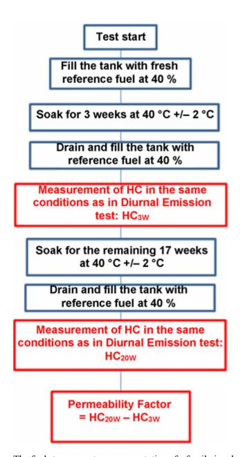
The fuel storage system representative of a family is selected and fixed to a rig, then soaked with E10 reference fuel for 20 weeks at 40 °C +/- 2 °C. The orientation of the fuel storage system on the rig has to be similar to the original orientation on the vehicle.
