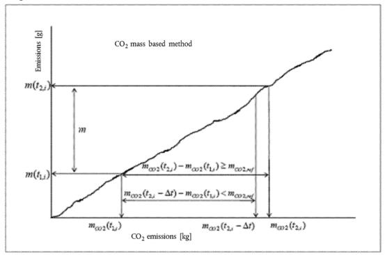
The duration  $(t_{2,i} - t_{1,i})$  of the i<sup>th</sup> averaging window is determined by:  $m_{CO2}(t_{2,i}) - m_{CO2}(t_{1,i}) \ge m_{CO2,ref}$
